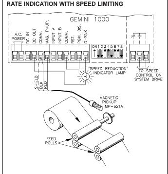
In this application, a GEMINI 1000 is used to indicate the speed of a printing press operation in feet/minute, while limiting the maximum speed to a desirable level.
