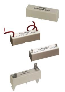
Very high isolation voltages, up to 15kV, are achieved through the use of high vacuum reed switches with either Rhodium or Tungsten contacts and make these relays suitable for high reliability applications, such as cardiac defibrillators, test equipment and high voltage power supplies.
