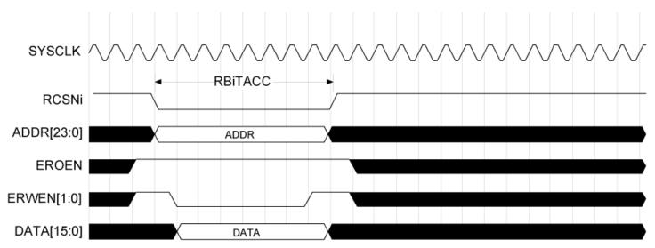
Figure 18. Static Memory Write Cycle
