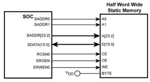
Figure 4. Static Memory Interface Examples
