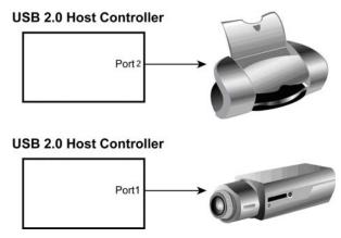
Figure 12. USB 2.0 Configuration as Two-Port Host
