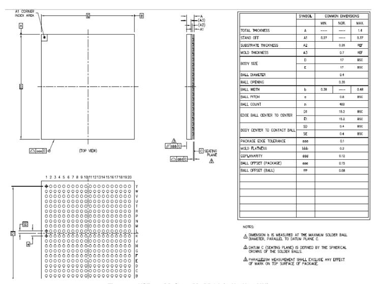
Figure 22. KSZ8692PB-S 400-Pin PBGA (17X17X1.4 MM)
