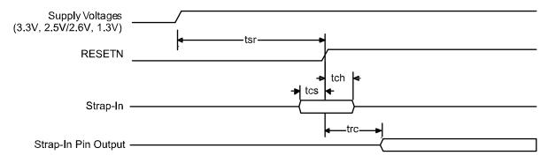
Figure 16. Reset Timing
