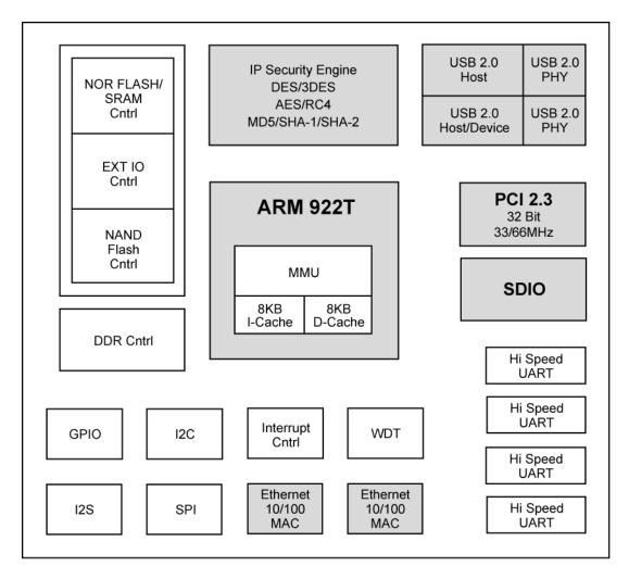
Figure 1. KSZ8692PB, KSZ8692PB-S Block Diagram
