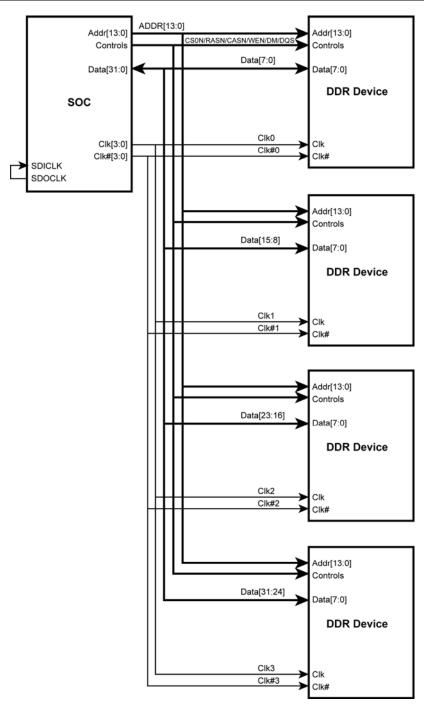
Figure 9. Four8-bit DDR Memory Devices Interface Example
