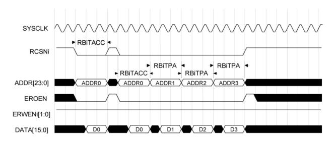
Figure 17. Static Memory Read Cycle
