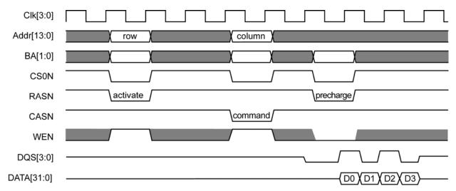
Figure 10. Burst DDR Read Timing
