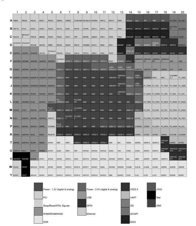
Figure 20. Ball Grid Array Map
