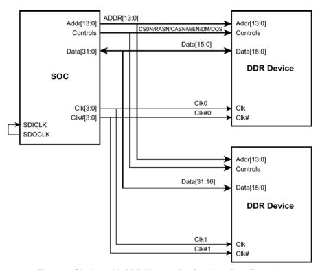
Figure 8. Single 16-bit DDR Memory Devices Interface Example
