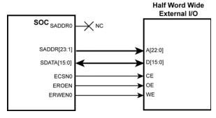
Figure 5. External I/O Interface Examples
