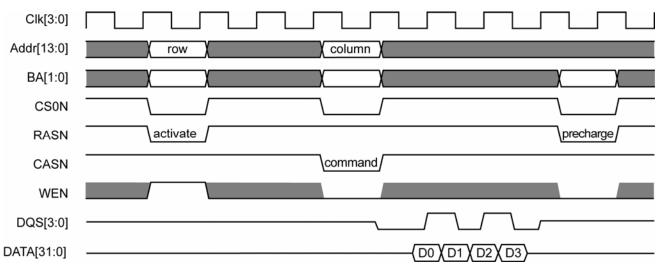
Figure 11. Burst DDR Write Timing
