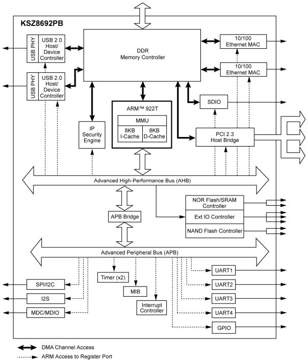
Figure 3. KSZ8692PB, KSZ8692PB-S Functional Block Diagram
