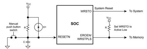
Figure 14. Reset Circuit
