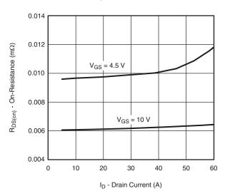
On-Resistance vs. Drain Current and Gate Voltage
