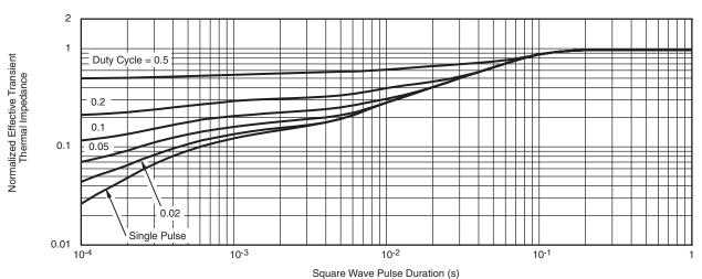
Normalized Thermal Transient Impedance, Junction-to-Source
