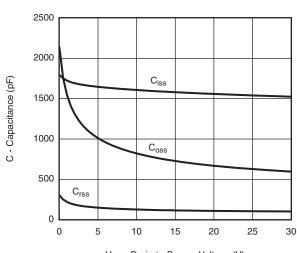
$V_{DS}$  - Drain-to-Source Voltage (V) **Capacitance**
