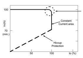
Typical LED power supply I-V curve
