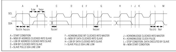
Figure 17. SMBus Read Timing Diagram
