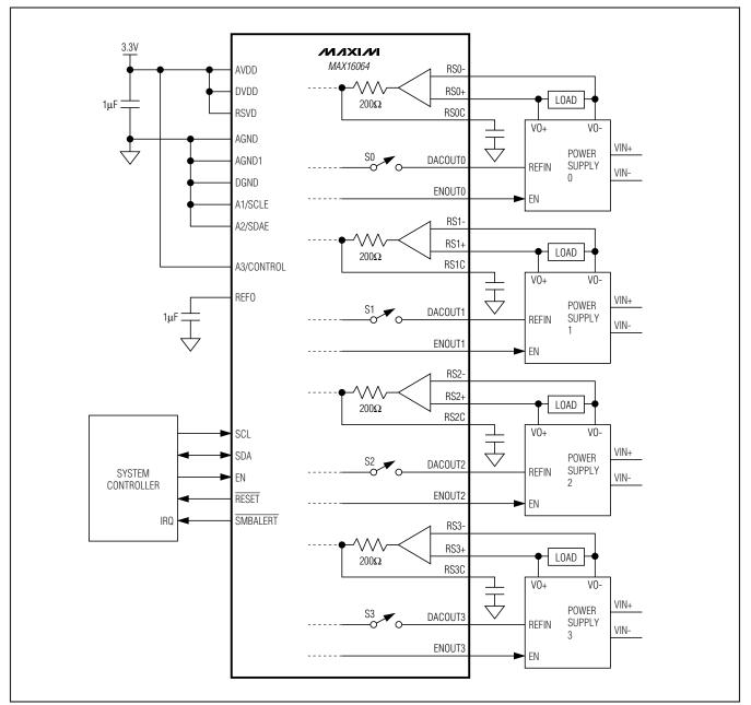
Figure 3. Typical System Application—REFIN Mode
