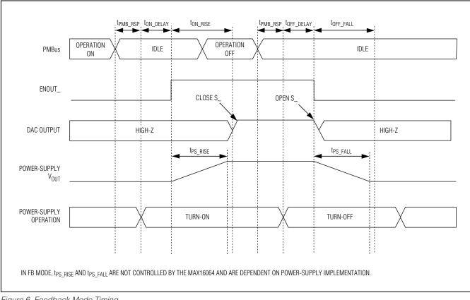
Figure 6. Feedback Mode Timing
