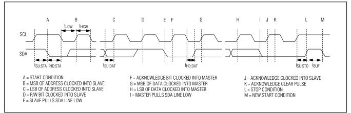
Figure 16. SMBus Write Timing Diagram
