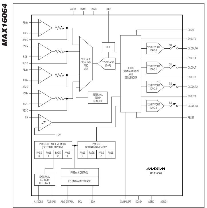
Figure 1. MAX16064 Functional Diagram
