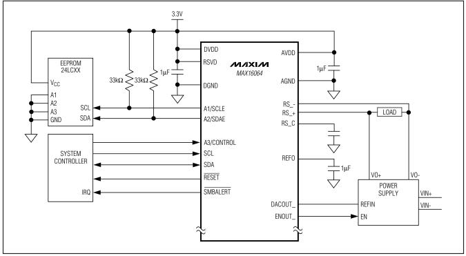
Figure 7. Typical System Application with External EEPROM
