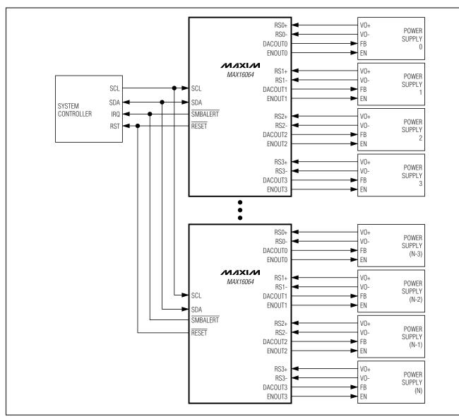
Figure 2. System Application Showing Multiple MAX16064s Controlling Power Supplies
