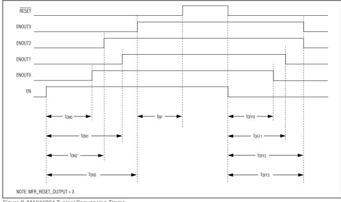
Figure 9. MAX16064 Typical Sequencing Timing
