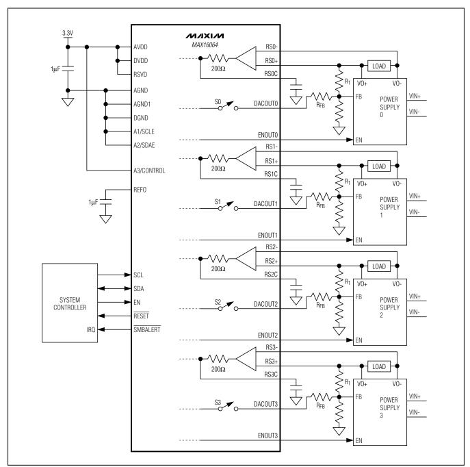
Figure 5. Typical System Application—Feedback Mode
